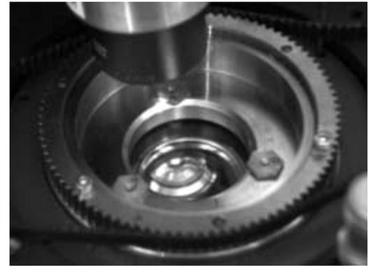
Fig. 4: Adjusted shear cell between illuminating condenser (top) and objective with central stop at the top (middle). Also visible the toothed belt drive on the cock-wheel and the micro-meter screws to adjust for planarity.
